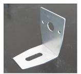
Fastwinch mounting bracket, 50L x 40W x 70H, 8mm slot for keel bolt, 13mm center hole 4mm bolt holes, 1.5mm or 2mm Aluminium COST \$10. available ex ChCh
