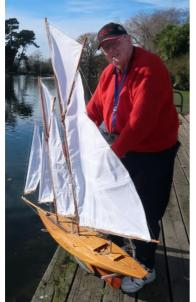
For the final finish on the deck and hull he applied five coats of two pot epoxy varnish. The Schooner carries 10lbs of lead in the keel. It has a two-channel radio and all sails are able to be trimmed together. Paul was delighted with the way she sailed.
