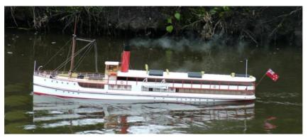
I decided to build the Earnslaw and try my hand at building a steam powered model. The model needed to be large enough to house the steam engine a boiler and a gas canister to fire the boiler.
