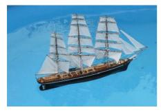
My next project was the Clipper Ship Cutty Sark. I had plans in a 1930s Model Engineer magazine and scaled them up to make an easy transportable fully rigged model over all 950mm long. Sailing conditions require fairly light winds, I have installed an electric motor and prop which helps going to windward.
