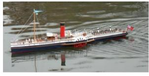
My latest project is the paddle steamer Bournemouth Queen, again the plans came from the Model Engineer. The model is 1130mm long propelled by a reversible electric motor which gives a realistic turn of speed.
