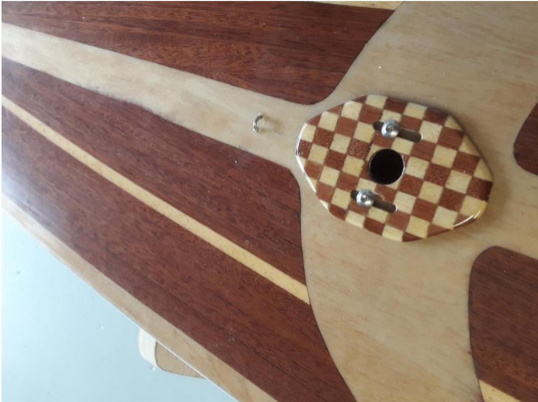
A close up of the finished deck, showing the planks and my custom chequer board mast ram.
